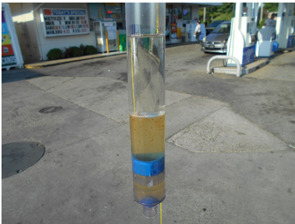
Sample from UST showing water with gasoline floating on top of it
